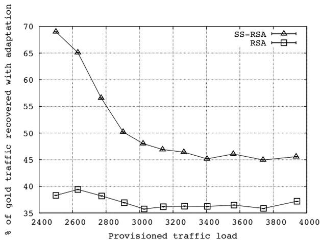
Fig. 3 Percentage of adapted gold traffic vs. provisioned network load.
