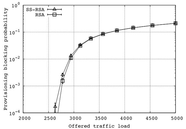
Fig. 4 Provisioning blocking probability vs. offered network load.
