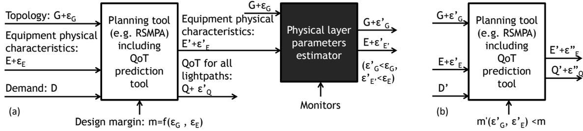
Figure 2: Design margin reduction with monitoring. (a) Training phase; (b) Estimation phase.
