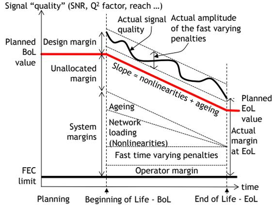
Figure 1: Margins and their evolution in a transport optical network.
